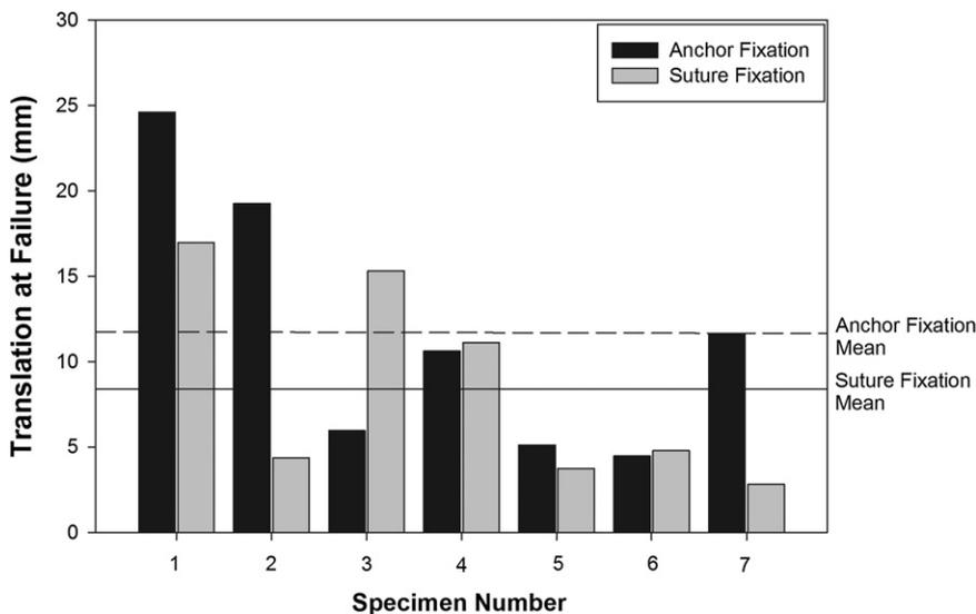
**FIGURE 4.** Translation at failure (in millimeters) of anchor versus suture fixation in 7 matched pairs of cadaveric shoulders.
